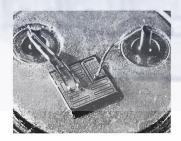
Because of past difficulties in bonding power semiconductor devices with large wire, manufacturers have used two or more small wires in parallel to provide current capacity. Extra wires were sometimes added to improve device reliability, the redundant wire providing an alternate connection in the event of primary wire
