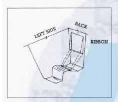
Orthodyne's ribbon tools are available for various ribbon widths and thicknesses, 1x5 to 3x30 mil. In conjunction with the Model 20R Ribbon Bonder, the tool is equipped with a guide slot to aid looping and positioning the ribbon. Tools for applications requiring special foot and groove configurations as well as tools without guide slots available. Consult the factory for specific information.
