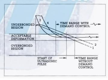
Curve 1 represents a bonding system with low sensitivity to loading by the bond (damping) as the bond interface increases. Curve 2 is the same system when surface films at the interface inhibit bonding.
