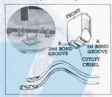
Type 4 is designed for bonding operations in which flying leads are required. Groove B (see figure), the cutoff groove, is oversize to avoid deformation of the wire as the cutoff ridge severs the wire lying on the nonbondable flat surface. The tool is ultrasonically vibrated during cutoff at a lower power setting than that used for conventional second bonds to achieve very clean cut ends.
